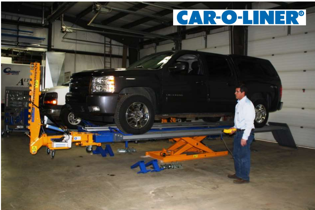
Car-O-Liner Bench Rack features push of a button electric pump. It also has removable ramps for easy access to the vehicle.
