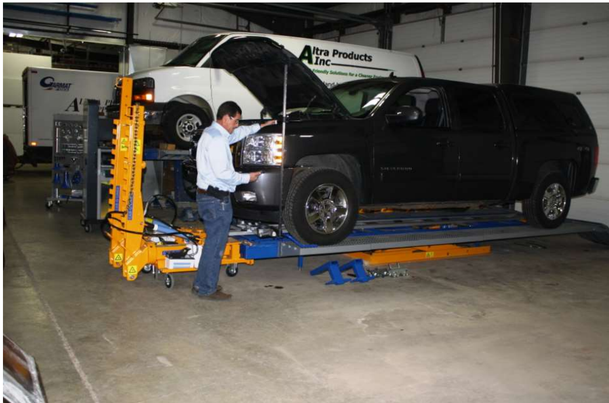
Car-O-Liner Bench Rack is easily used with the Vision computer measuring system. Vision X3 allows for smart phone monitoring of the measuring process.
