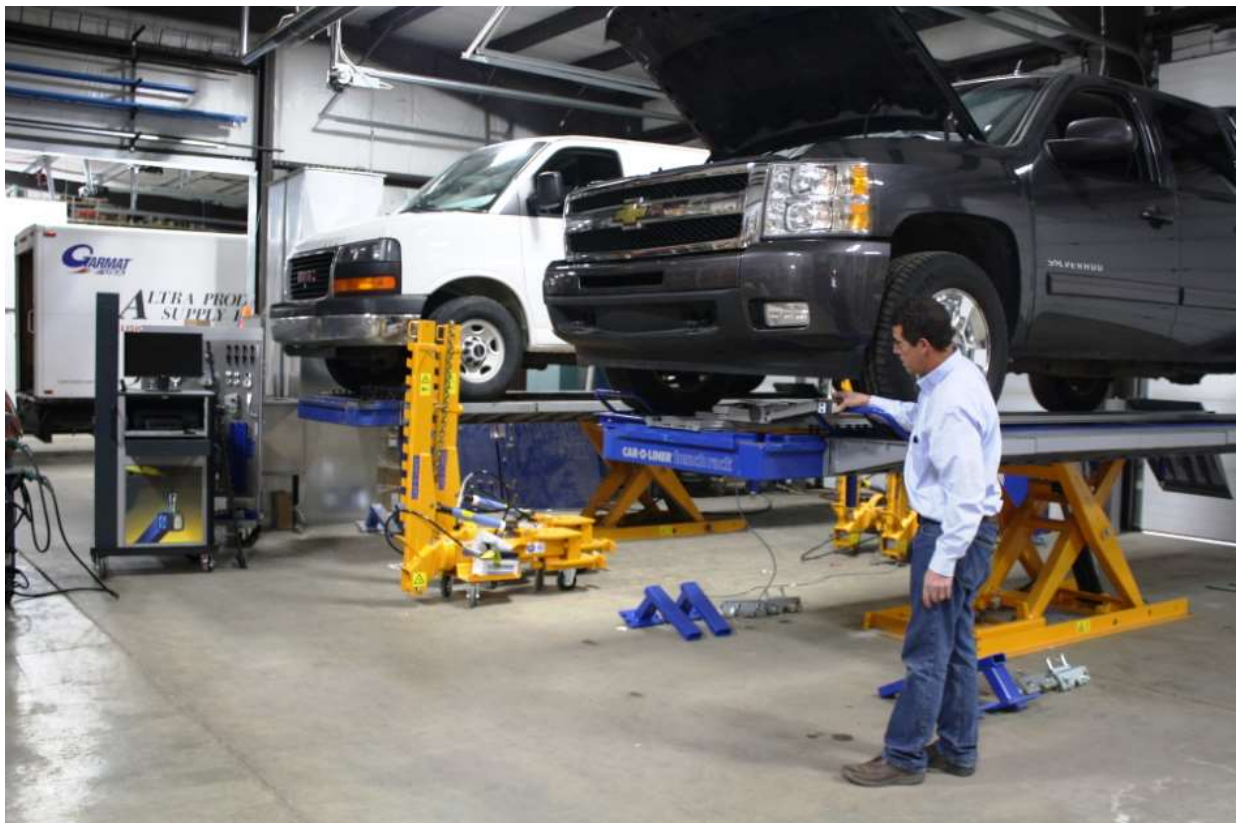
Car-O-Liner Bench Rack allows the technician to add or remove towers easily for all sorts of operations and repair procedures.
