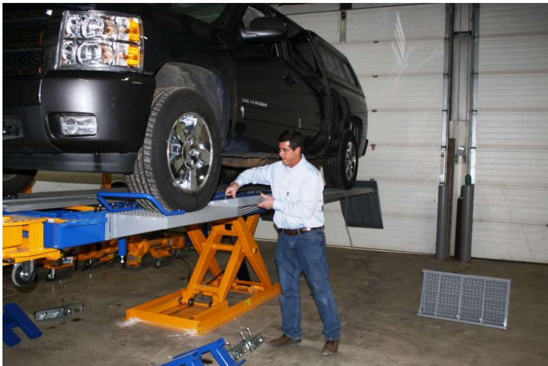
Car-O-Liner Bench Rack features push of a button electric pump. It also has removable ramps for easy access to the vehicle.
