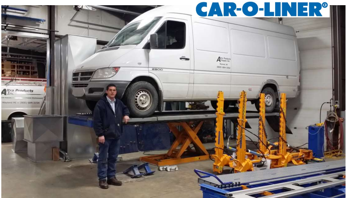
Car-O-Liner Bench Rack allows the technician the ability to repair small and large vehicles on the same platform, at any given heights to prevent fatigue. After all our technicians are getting older!
