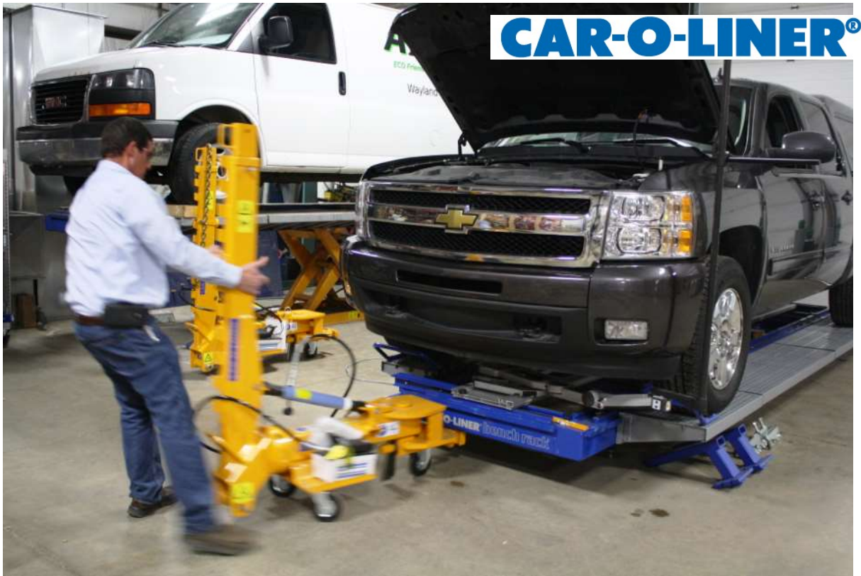
Car-O-Liner Bench Rack allows the technician to add or remove towers easily for all sorts of operations and repair procedures.
