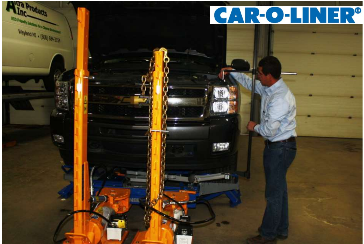
Car-O-Liner Bench Rack is easily used with the Vision computer measuring system. Vision X3 allows for smart phone monitoring of the measuring process.
