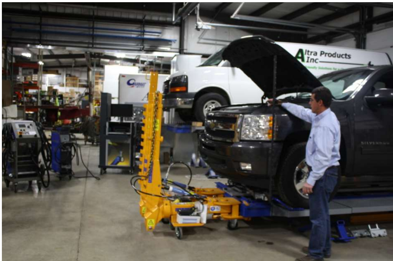
Car-O-Liner Bench Rack allows easy access to repairing all types of vehicles at any working height the technician chooses.
