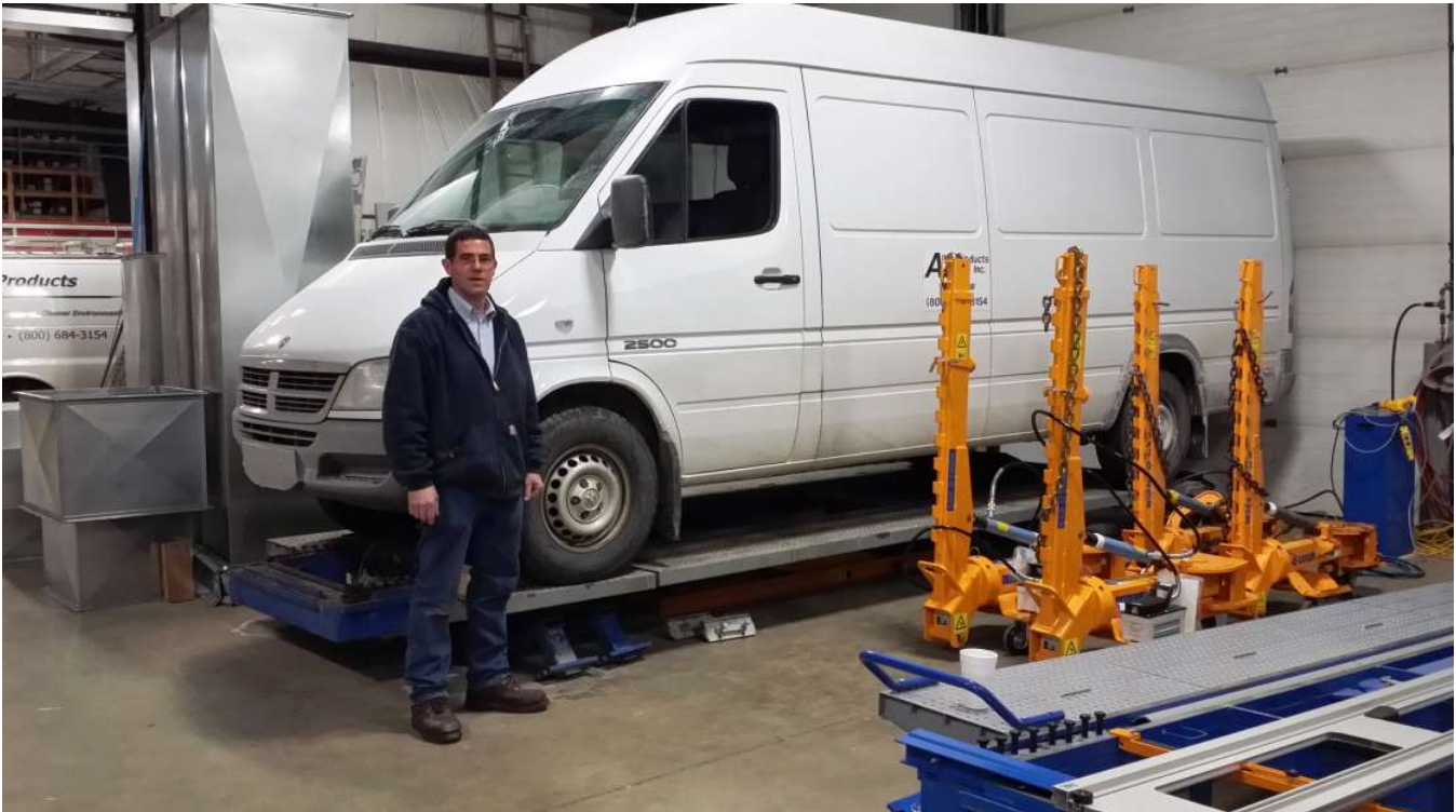
Car-O-Liner Bench Rack allows the technician the ability to repair small and large vehicles on the same platform, at any given heights to prevent fatigue. After all our technicians are getting older!
